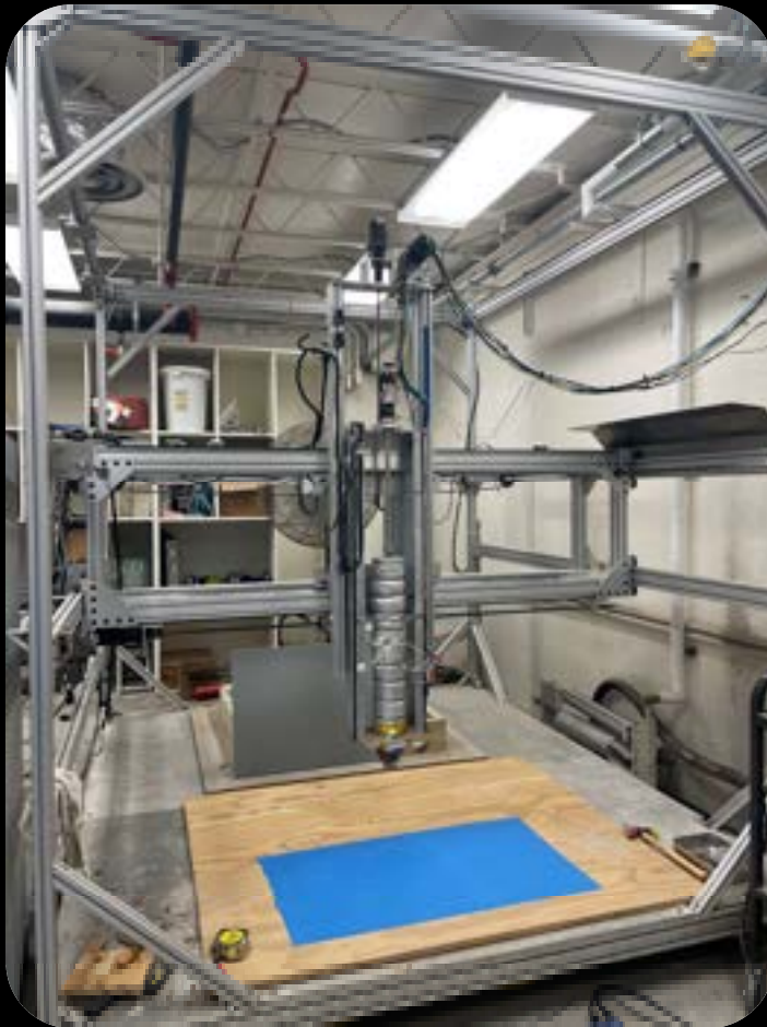
Plasma torch test extreme heat simulation for landing pads
